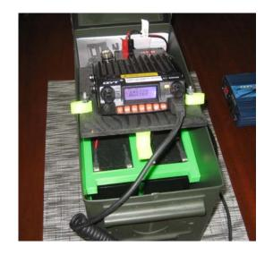
3D printed batterey brackets hold batteries in place during movement.
